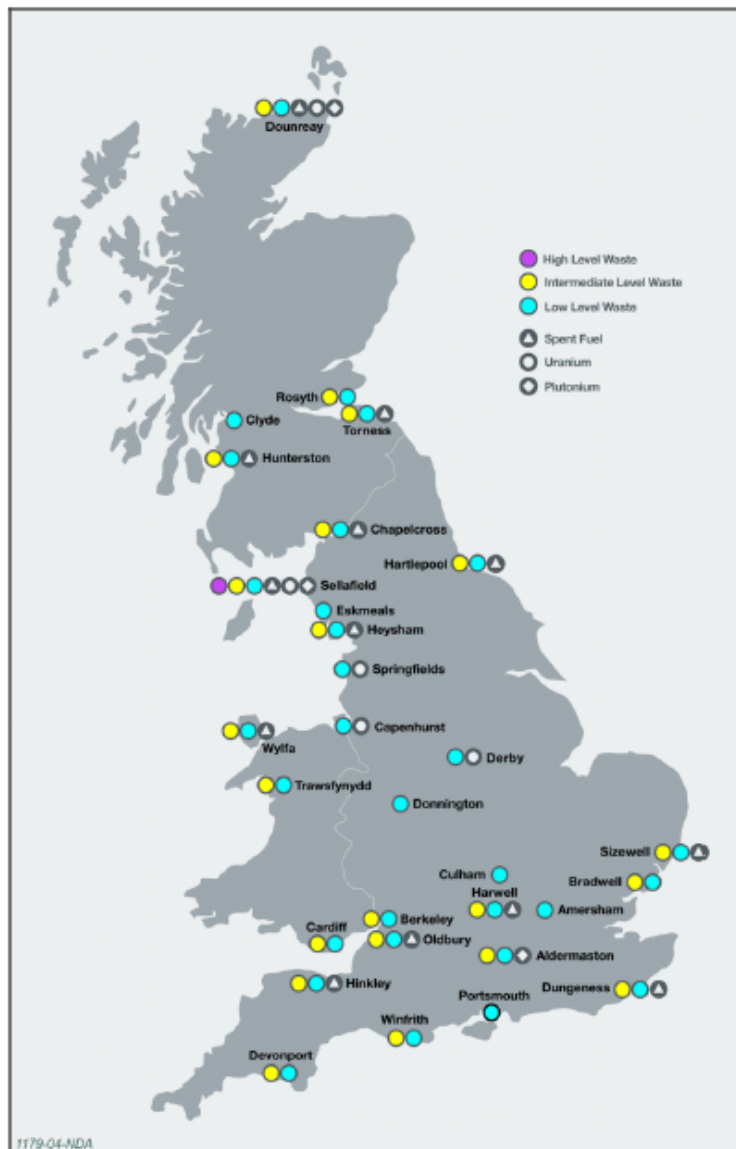
Figure 1.1. Sites where radioactive waste and materials are currently stored. Source: Taken from DECC (2014) (p. 16).
